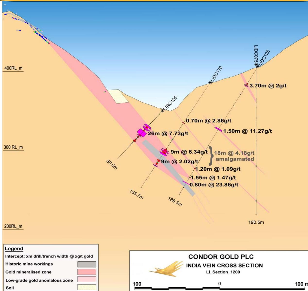
Cross section: example of historic mine workings, La India and California veins and limit of whittle open pit shell
