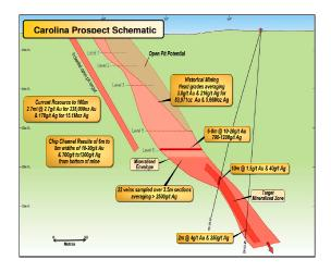
The mineralisation and alteration encountered within this trenching gave excellent confirmation of Condor's target model of broad stock work zones of gold mineralisation with inter-fingering high grade quartz veins. This suggests that open pit mining may be possible, with subsequent underground mining of higher grade mineralised zones.
