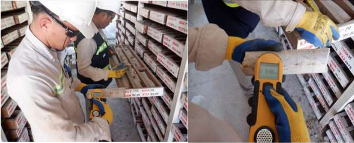
Figure 4. Photos of Condor's personnel collecting magnetic susceptibility from La India drill core.
