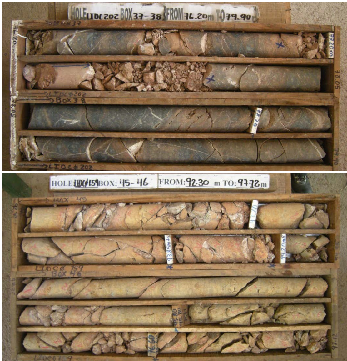
Figure 24-5: Hangingwall Core Intersections
