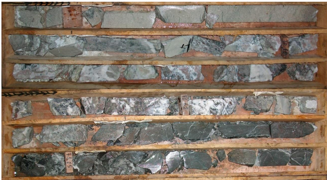
EODH-01: 6.87m (5.6 m true width) @ 0.66g/t Au from 65.53m drill depth, including 1.50m (1.2m true width) @ 0.89g/t Au from 65.53m and 1.2m (0.9m true width) @ 1.25g/t Au from 69.50m depth. Gold mineralisation of 2.40m @ 1.25g/t Au from 69.50m. Mineralisation is associated with quartz-calcite breccia at the contact between felsic (HW/South) and mafic (FW/North) rocks with the best grade on the mafic side of the contact. The breccia is strongly silica-haematite-chlorite-sulphide altered. The wallrock has chlorite-haematite alteration and fracture-fill quartz-carbonate-sulphide in the wallrock with very low grade gold (<0.1g/t).
