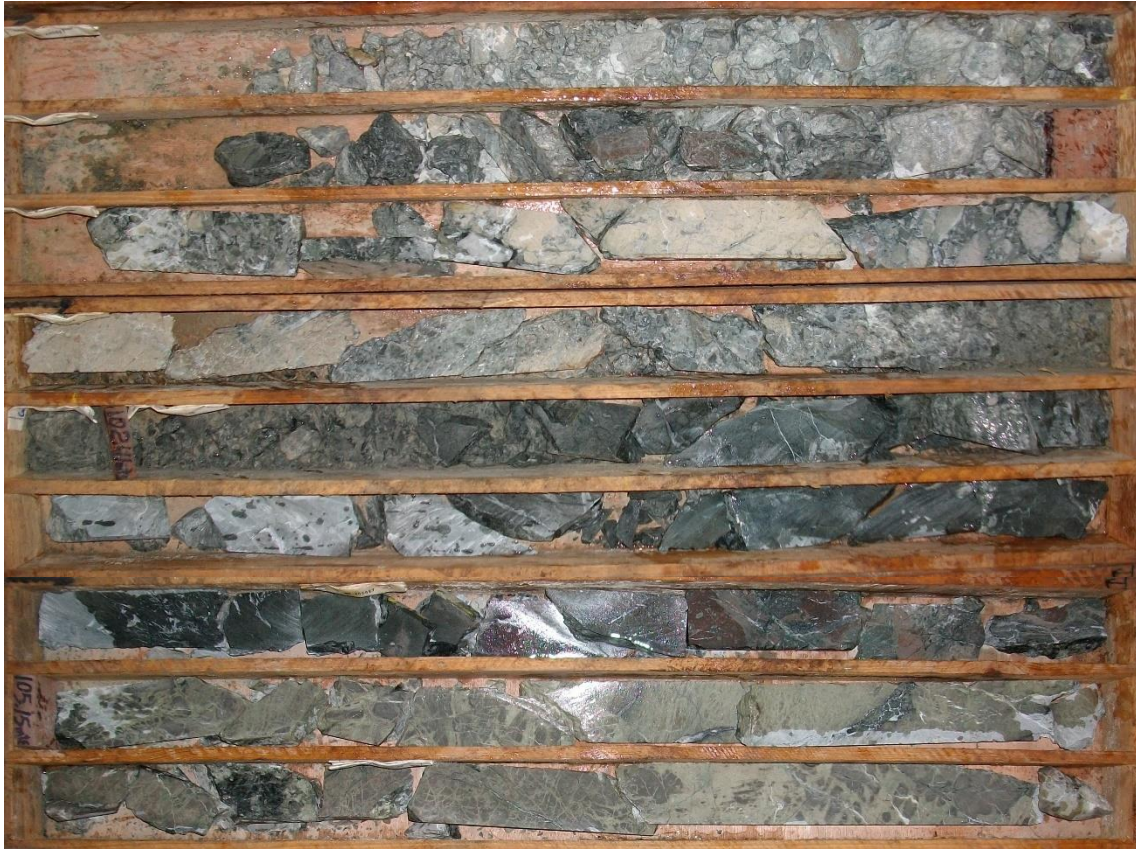
EODH-08-03: 14.53 m (8.3 m true width) @ 0.82 g/t Au from 83.32 m depth including three zones grading up to 1.8 m (1.0m true width) @ 2.38g/t Au. The mineralisation is associated with a stockwork of fracture-filling quartz-calcite veins hosted by felsic rock (tuff) and felsic lapilli tuff near the contact with mafic rock.
