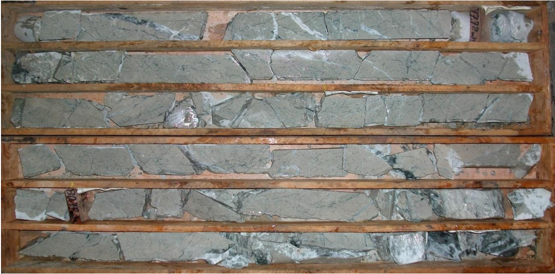
Quartz-calcite-chlorite-sulphide veining and haematite alteration in drill hole EODH-08-03: 14.53 m (8.3 m true width) at 0.82 g/t from 83.32 m.
