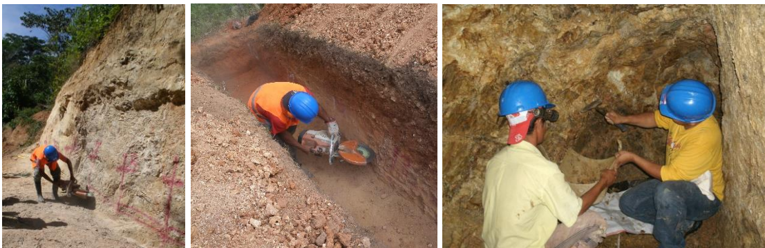
Figure 9. Channel sampling by Condor in 2011 at the historic Estrella Mine: face sampling (ESCT001; left), trenching (ESTR1; centre) and underground in the historic mine (ESTN001; right).
