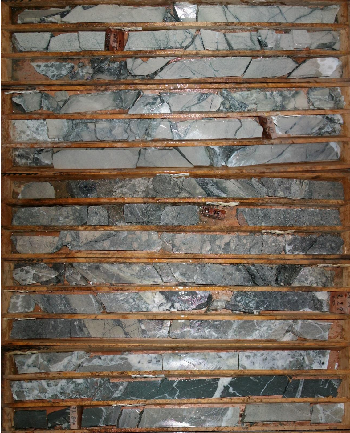
EODH-08-02: 6.50 m (5.3 m true width) @ 1.64 g/t g/t Au from 65.50 m is a breccia zone, possibly a volcanic breccia overlying a thin (2-3 m) mafic unit. Gold mineralisation is associated with replacement and fracture-fill quartz-carbonate veins. Gold mineralisation improves towards the base with 4.25 m (3.5 m true width) @ 2.24 g/t Au. Alteration is strong chlorite-carbonate-sulphide concentrated in the mafic rocks.
