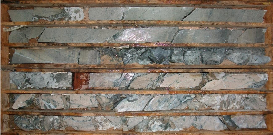
EODH-08-02: 1.20m (1.0m true width) @ 1.50g/t Au from 43.00m 1.2m (0.8m true width) showing intense silica-carbonate-haematite alteration of a felsic protolith.
