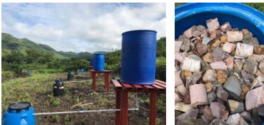
Kinetic field test (left) and core samples in one of the reactors (right)
